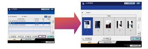
Preview function makes it possible to check the scanned image instantly on the control panel. You no longer need to return to your PC to check the scanned data. If necessary you can redo scans at the e-STUDIO. In the e-STUDIO4540CSE series, this function became available on the **Scan and FAX functions**. In addition, you can replace, add and delete a page on scan preview function.
